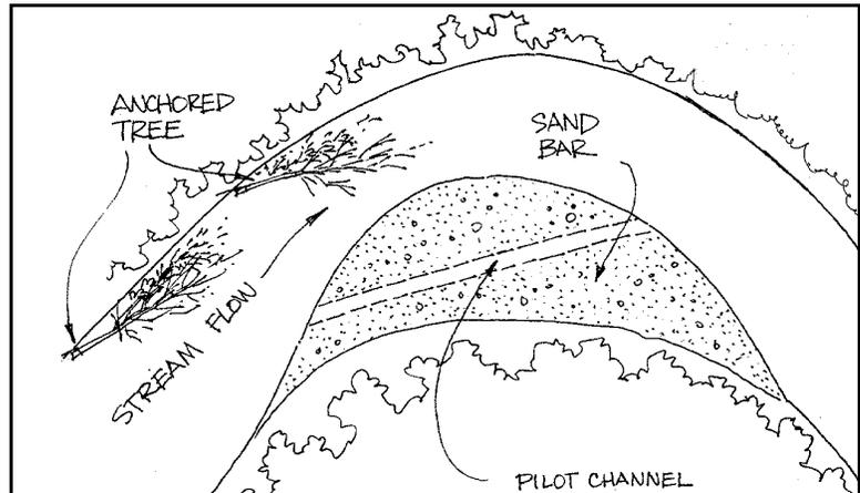
Exhibit 403d: Felled trees anchored to the streambank deflect flows away from the bank to prevent erosion (Source: Ohio Stream Management Guide)
